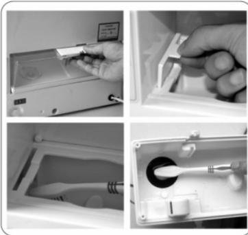
Use citric acid detergent and follow the instructions to configure solution, pour into the humidifier and soak for 10-20 minutes, then use the toothbrush or cloth to clean the humidifier, discharge the water through the outlet, and then rinse one more time.
