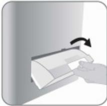
**1** Press and hold the water tank clasp at 45 ° and remove the water tank.
