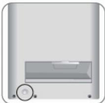
**5** When the humidifier is not in use, discharge the water from the water outlet and keep the water tank empty.
